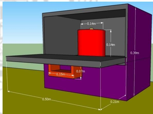
The Manual Robot will give a slight touch to the door using the handle, so that door falls outside and Manual Robot will take The Uri Handler placed inside.
