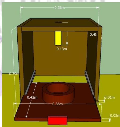
The Manual Robot will place the Wired Bomb in the cavity and push the red handle so that it slides the plank inside.
