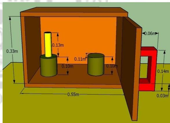
The Manual Robot will take the two bombs (Wired and Non-Wired) by opening the door using the handle.
