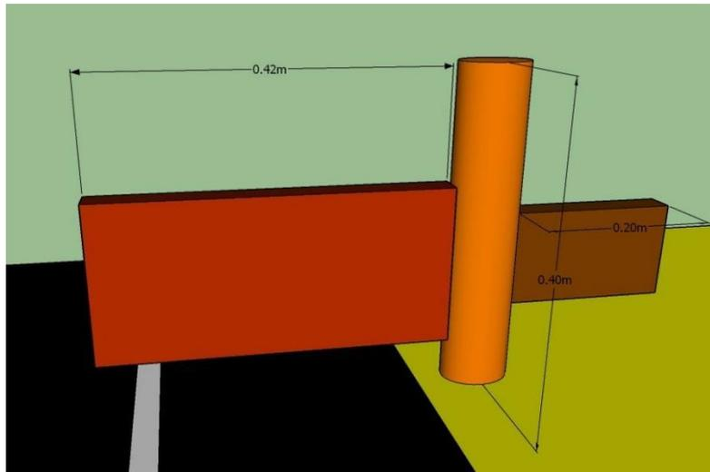
The Manual Robot will rotate the Line Of Control Gate (extended in Manual Robot's Arena) such that the part of the gate in Auto Robot's arena rotates to clear the path of Auto Robot.
